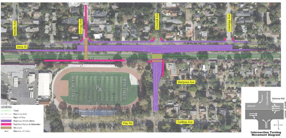
Figure 3 Churchill Partial Underpass Alternative
