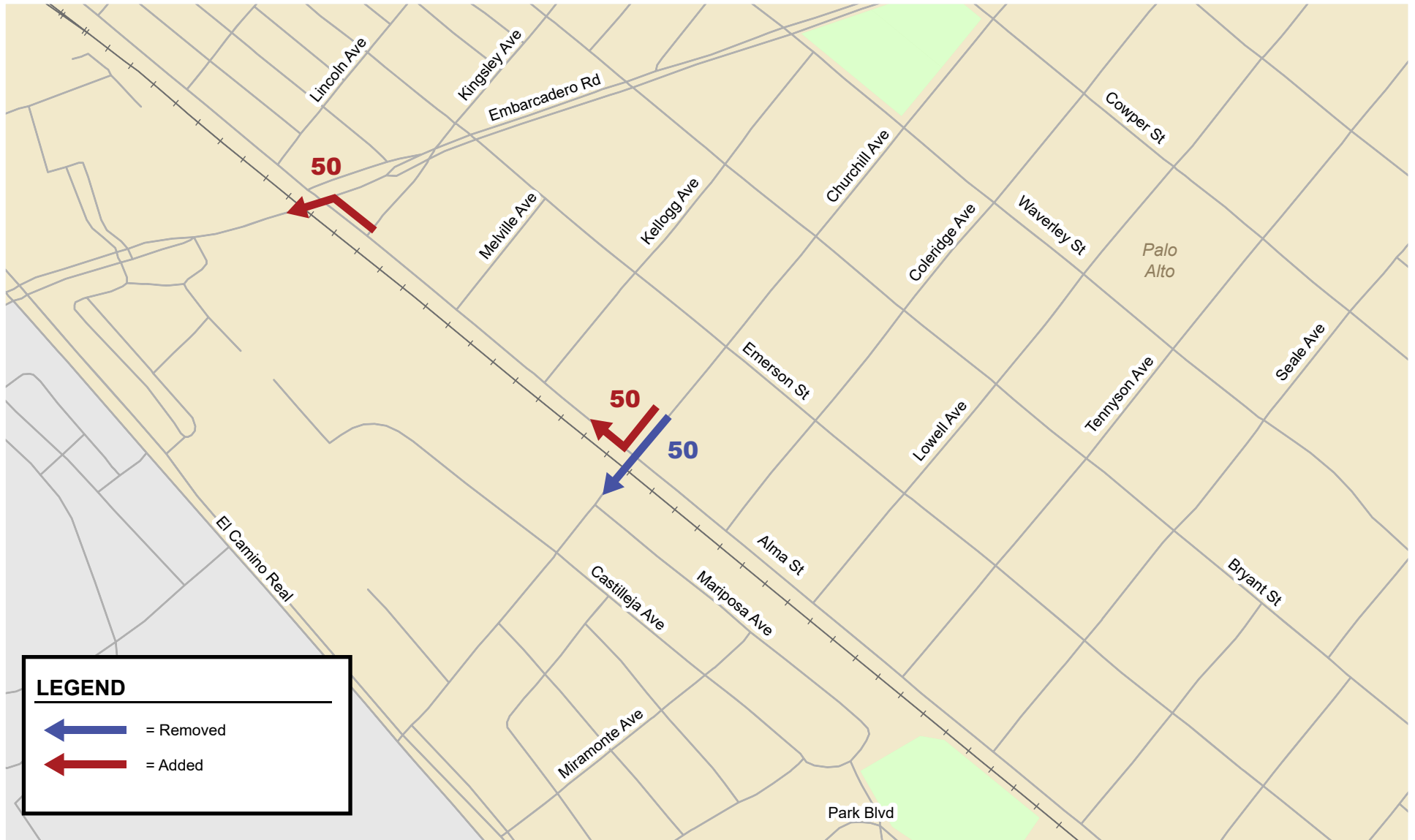
Figure 4B Churchill Ave/Alma St AM and PM Peak-Hour Diversions (Partial Underpass Alternative)
