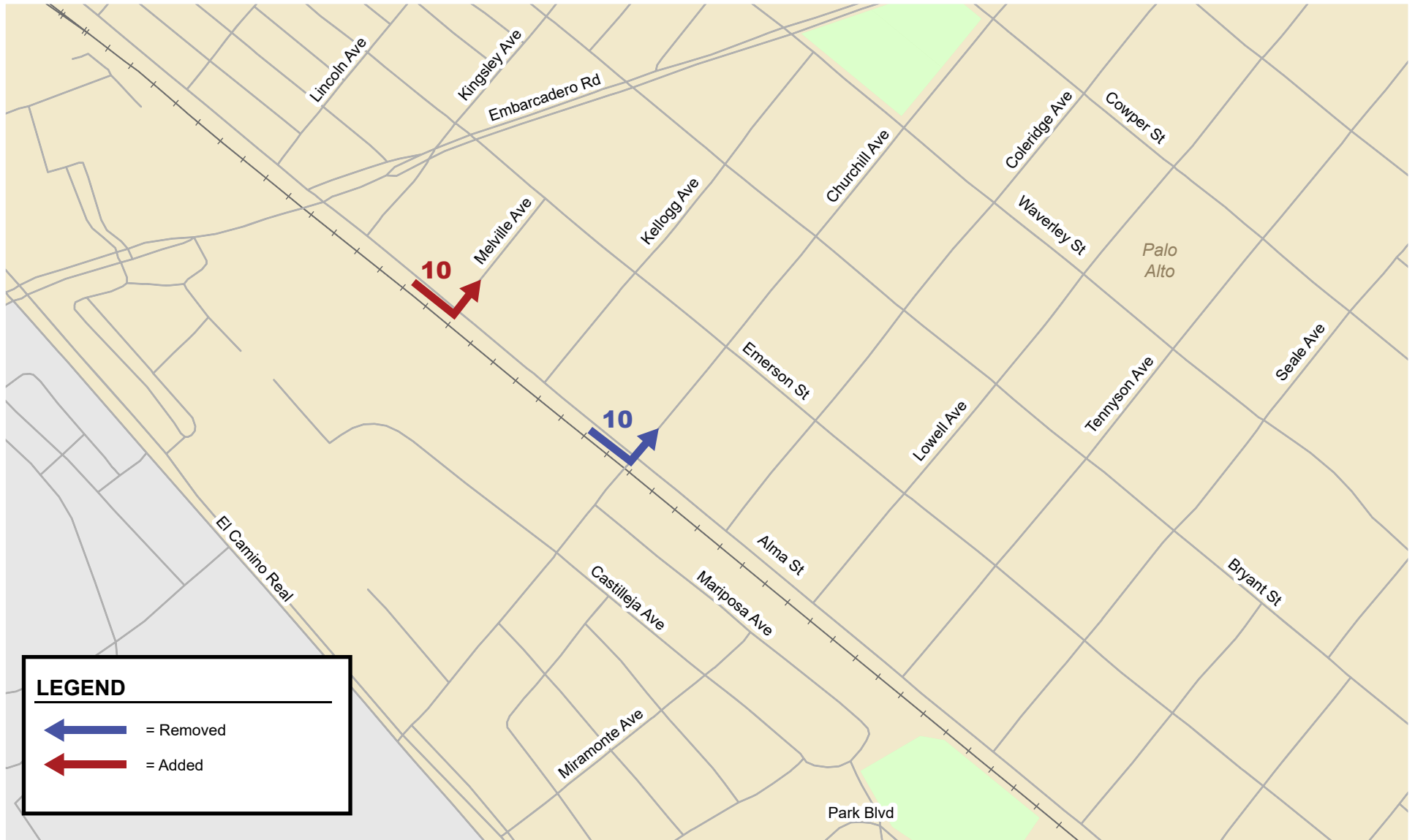
Figure 4D Churchill Ave/Alma St AM and PM Peak-Hour Diversions (Partial Underpass Alternative)
