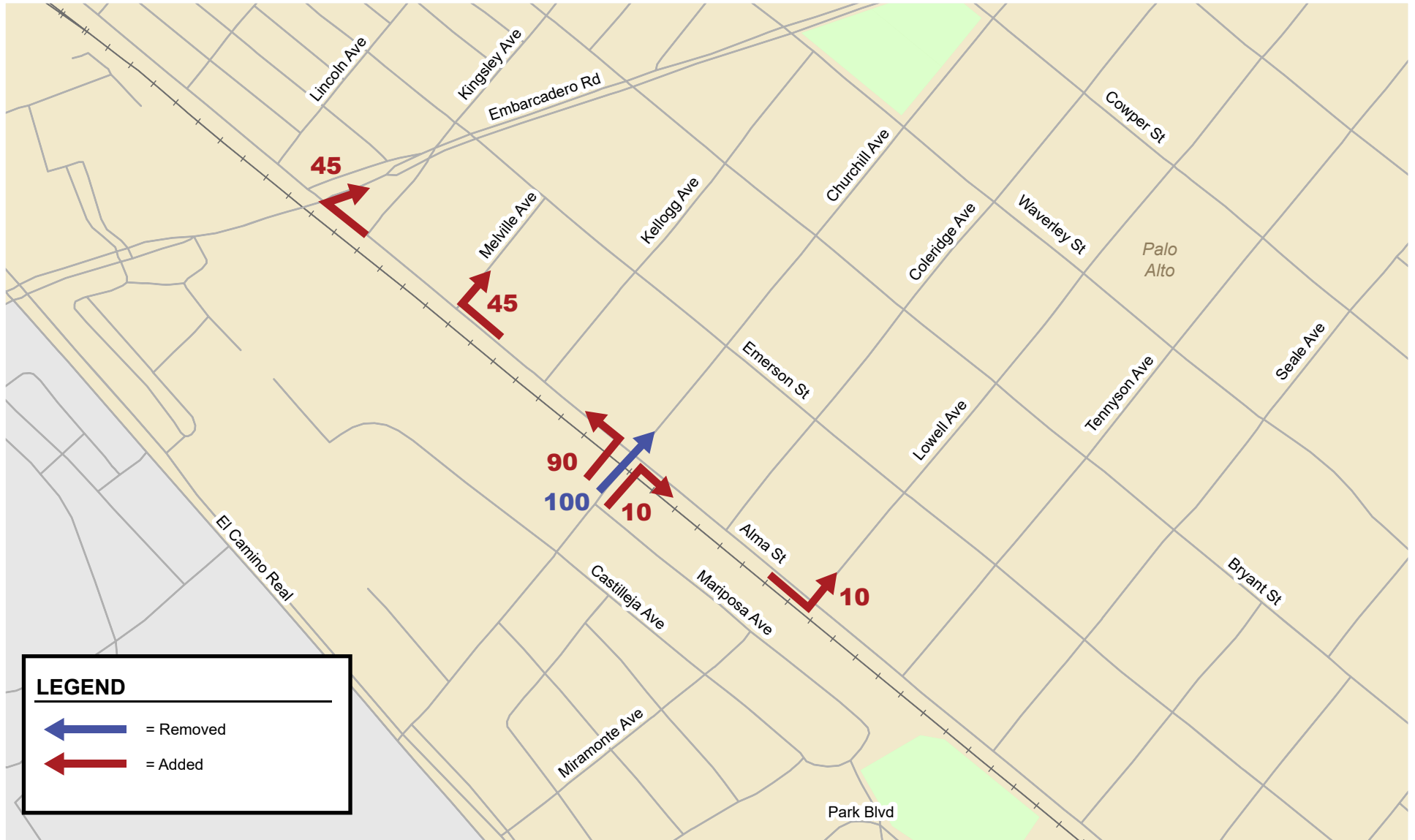
Figure 4A Churchill Ave/Alma St AM and PM Peak-Hour Diversions (Partial Underpass Alternative)
