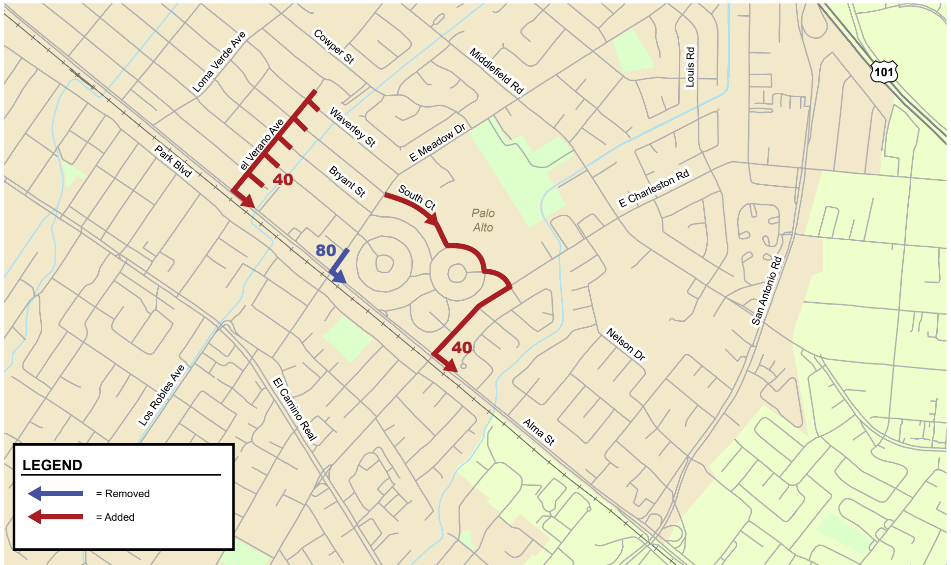
Figure 9A E Meadow Dr/Alma St AM and PM Peak-Hour Diversions (Partial Underpass Alternative)
