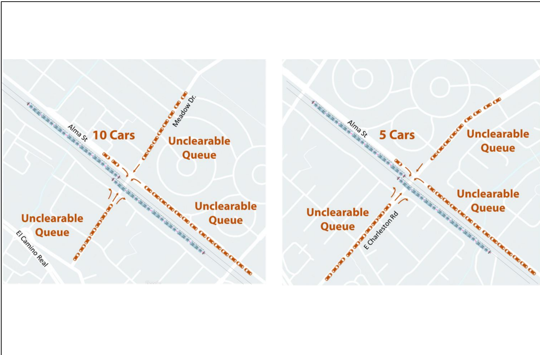
Figure 5.4 2030 PM Peak Period Estimated “No Build” Queues at Meadow Dr. & Charleston Rd.
