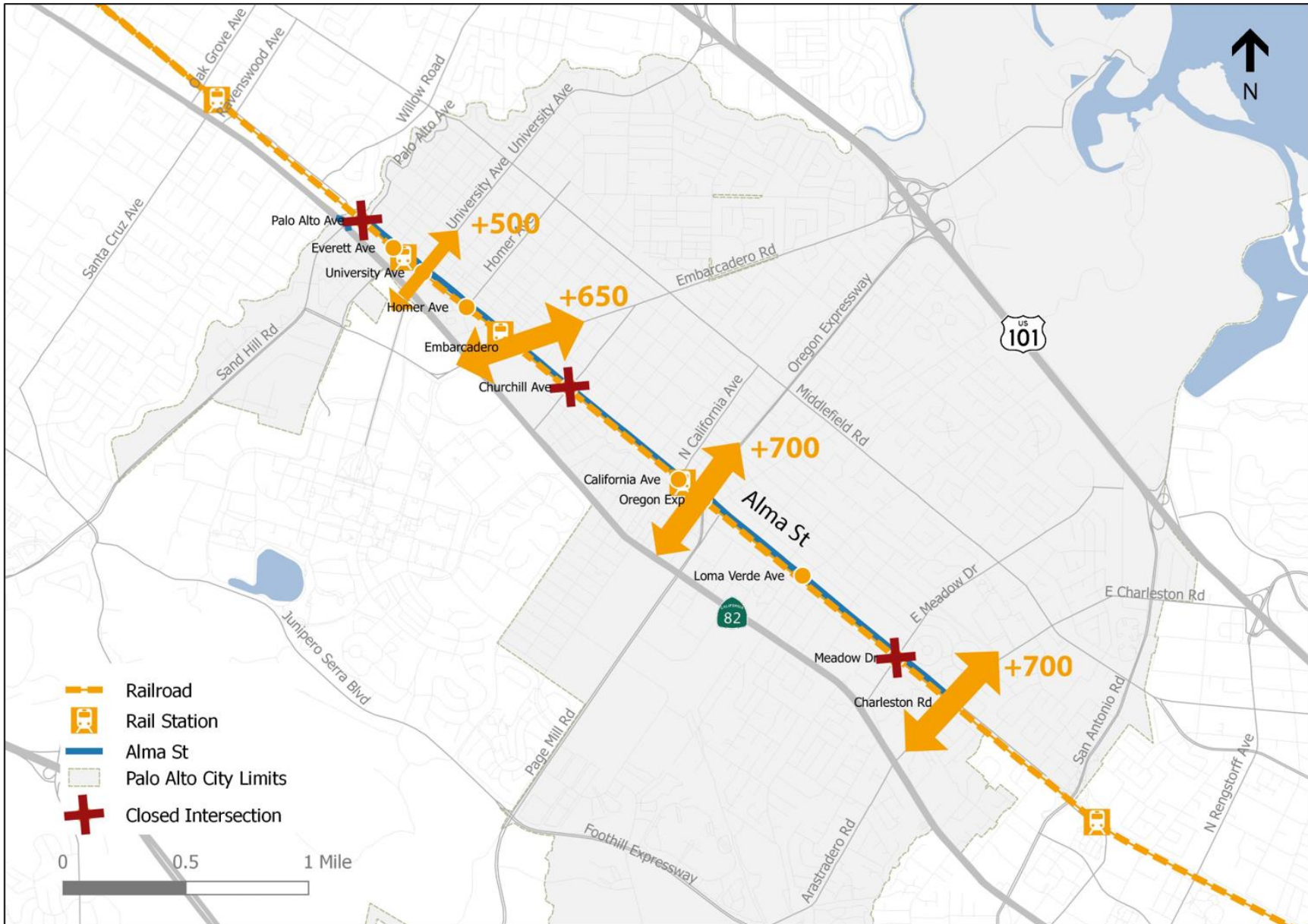
Figure 4.13 Flow Increases From 2017 to 2030 (AM Peak) VPH: All At-Grade Closed Except Charleston Rd. – Sample Scenario 1
