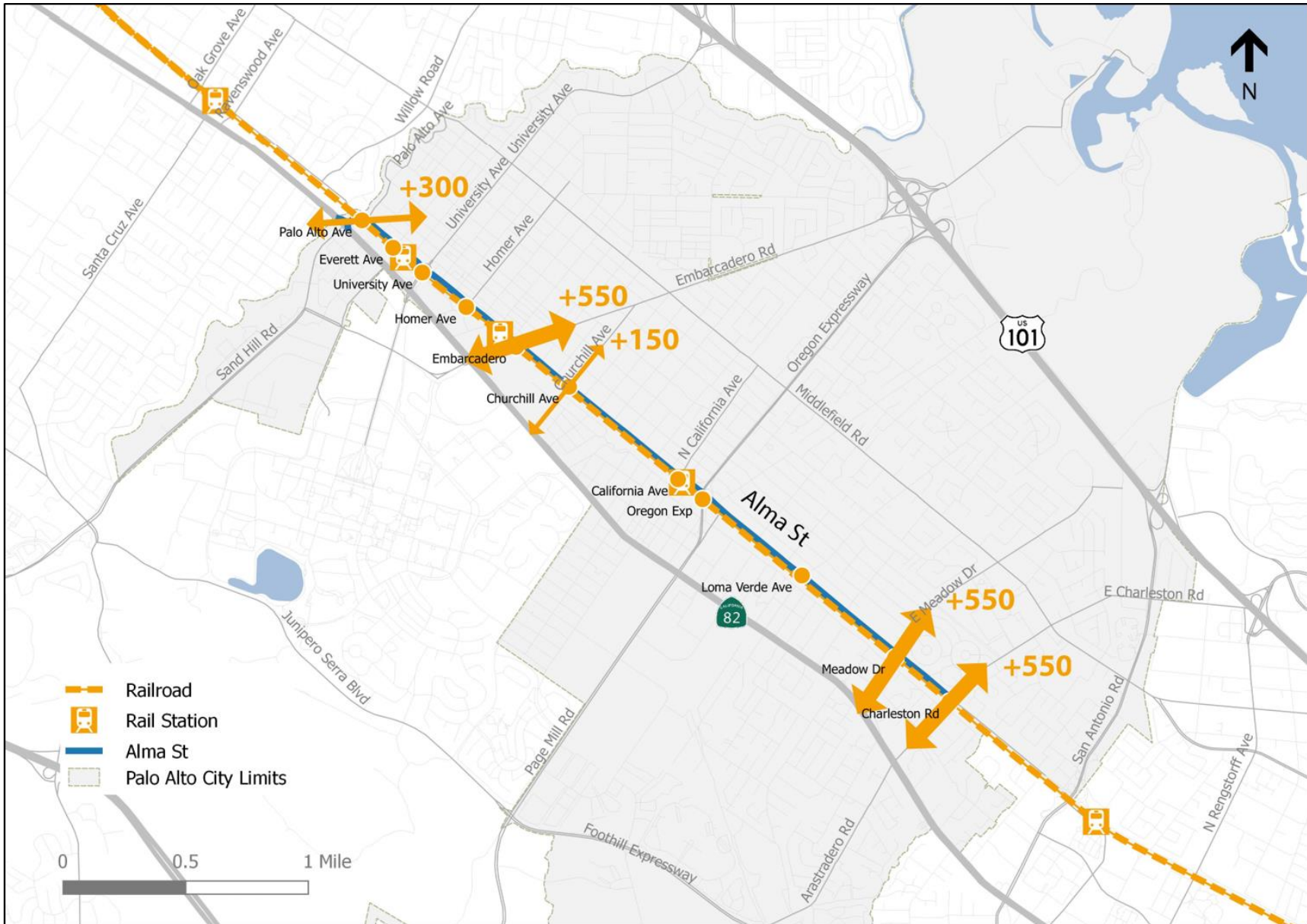
Figure 4.15 Flow Increases From 2017 to 2030 (AM Peak) VPH: Full Grade Separation Except Churchill Ave. – Sample Scenario 6
